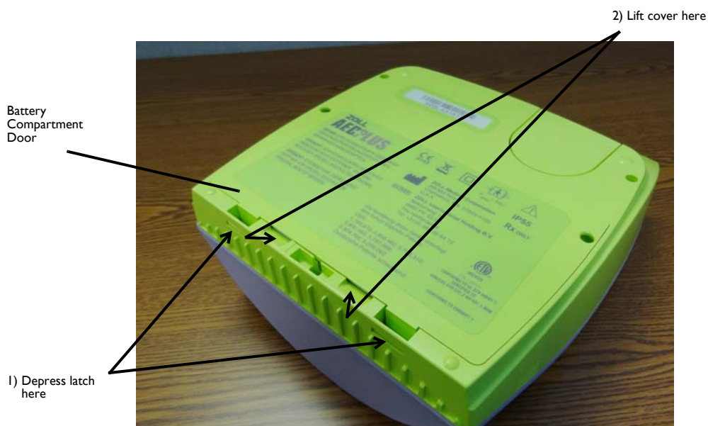
Figure 7: Removing the Battery Compartment Door
